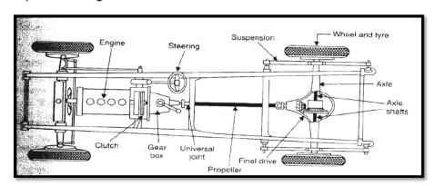
It contains the source of power, i.e. engine, the frame, which supports the engine,
