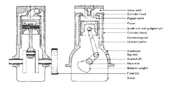
The description of main components of IC engine is given below:
